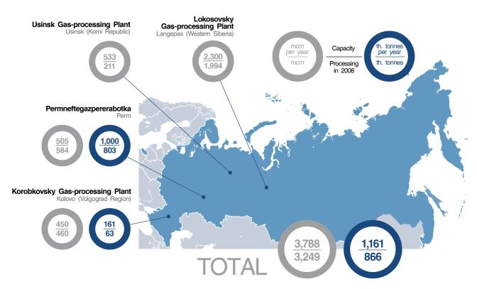
Gas-processing plants of LUKOIL Group process associated gas from fields in Russia into marketable gas (fed into the Gazprom gas pipeline system) and liquid hydrocarbons.
