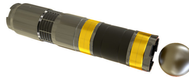
A pump-down plug is used to isolate hydraulic fracturing stages. The design of the plug allows it to be pumped into the well using a connected pump. The large flow area of the plug ensures uninterrupted operation of the well. If necessary, it is possible to drill through the plug, since it is made of composite materials.
